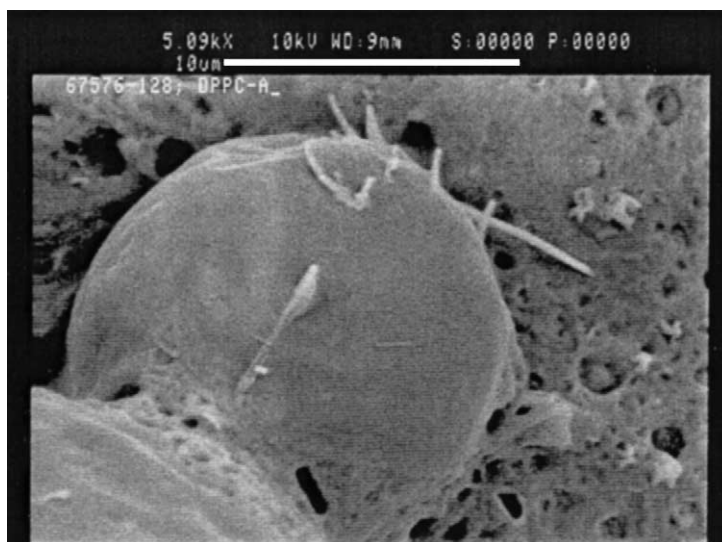
Fig. 1. SEM picture of a liposphere formulation containing 3% bupivacaine, 6% tristearin, and 3% DPPC.
